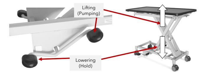
For lowering the table top, press the left (shorter) pedal. When doing so, however, it is necessary to push this pedal and hold it down until the table top has again reached the desired height. Releasing the pedal brings the table top to a standstill at the desired height.
